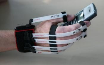
Fig. 2.19: Cambridge simulation gloves: The gloves limit the strength and range of movement of the fingers and thumb. (inclusivedesigntoolkit.com/tools simulation/)
