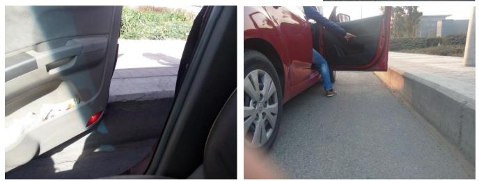
Fig.2.10: An extremely elevated sidewalk than the street level urges a car driver to stop far away from the sidewalk.
